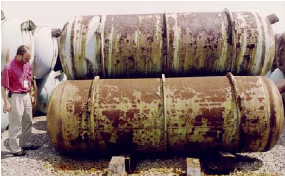
Depleted uranium storage cylinders at the Portsmouth (Ohio) Gaseous Diffusion Plant site. (U.S. DOE)
